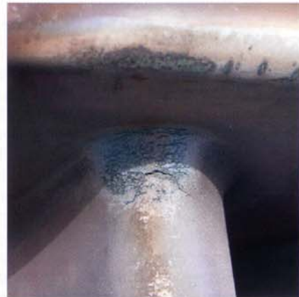
2-2. Onsite inspection identified the need to repair this Model 7FA second-stage nozzle (above)
