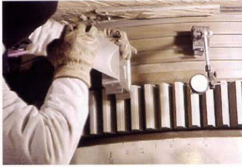
1-3. Slow rotation of the turbine rotor causes blades to “rock,” opening clearances between blade roots and mating rotor slots. Blade rock should be measured during or prior to disassembly (left)
